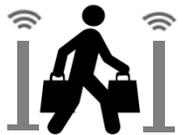
When the customer goes through the RFID gate placed at the exit of the store, the system accurately identifies the items. In case of theft, it activates the alarm.
